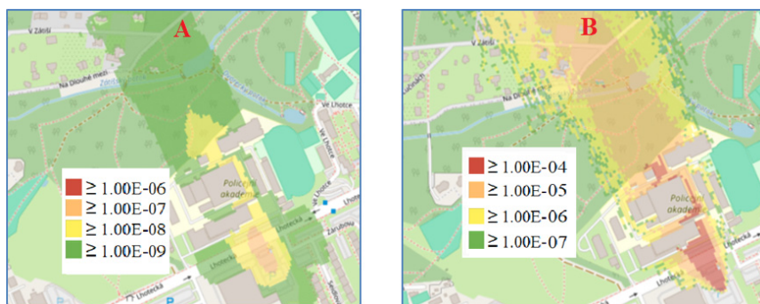
Fig. 3. An example of spreading radioactive cloud Cs-137 of original activity of 10^{12} Bq close to the campus of PA CR in terms of external radiation (A) and committed effective dose (B) in Sv during the first 10 min after the release. [2]
